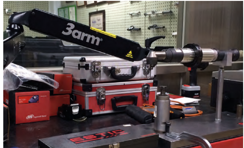
A compact multi-purpose arm for use when brakes are not required
